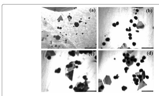
Figure 5 Characterization of AuNPs formed with 1 mM chloroauric acid and 5 % GGFE at 40°C by transmission electron microscopy (TEM). (a) Anisotropic gold nanotriangles; (b) Gold nanotrapezoids; (c) Gold nanospheres and triangles with equilateral edges; (d) Gold nanotrapezoids and spherical nanoparticles adsorbed on surface of triangles. The inset bars represent 200 nm.
