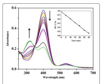
Figure 11 Time dependent UV–vis spectra for monitoring 4-nitrophenol reduction by NaBH<sub>4</sub> catalyzed by AuNPs. The inset shows the plot indicating the variation of  $\ln (A_t/A_0)$  vs time.
