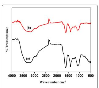
**Figure 10** FTIR absorption spectra of dried GGFE before bioreduction (a), after complete bioreduction at 50°C (b) of chloroaurate ions.
