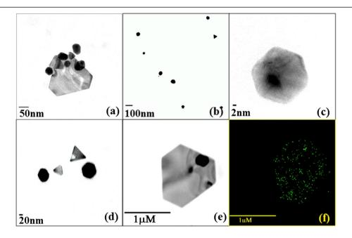
**Figure 6** Characterization of AuNPs formed with 1 mM chloroauric acid and 5 % GGFE at 40°C by high resolution transmission electron microscopy (HRTEM). (a) Anisotropic AuNPs adsorbed on surface of each other; (b) Spherical nanoparticles in a range of 10 nm.; (c) Gold nanohexagon with equilateral edges; (d) Gold nanotriangles and hexagons; (e) Scanning transmission mode micrographs for gold nanotrapezoid; (f) Elemental mapping of gold nanotrapezoid.
