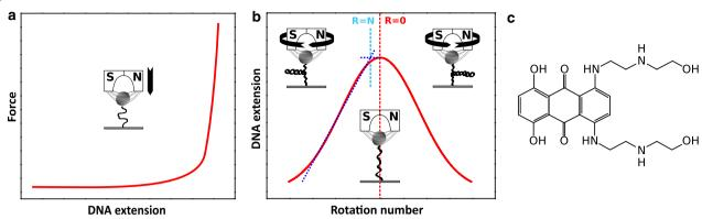
**Fig. 1** Schematic of the MT assays for **a** extending and **b** overwinding a single dsDNA molecule (hat curve). Blue dashed lines divide the hat curve into two regions where a dsDNA polymer exhibits different torsional behaviors. The rotation number at the transition point is referred to as buckling number (for details see main text); **c** chemical structure of MTX
